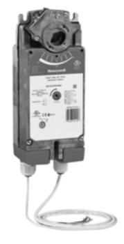
Actuator Type: Damper; Valve Rotational Stroke: 95 ±3 degrees Fail Safe Mode: Spring Return Torque Rating: 175 lb-in. (20 Nm) Spring Return Torque: 175 lb-in. (20 Nm) Spring Return Direction: By orientation
