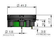
All dimensions in mm All tolerances ±0.15 mm unless otherwise stated 3SF shown with side tags and tin pins
