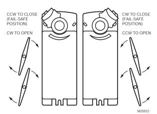
Fig. 2. Spring Return DCA mounting orientation.
