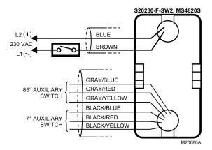
Fig. 11. Typical 230 Vac wiring (S20 Series).
