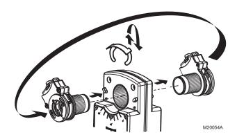
Fig. 4. Mounting shaft coupling to actuator opposite
