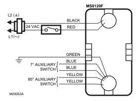
Fig. 7. Typical 24 Vac wiring (MS Series).
