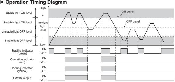
%The above diagram is the state of operation for Light ON, but in case of Dark ON, it is opposite operation against Light ON.
