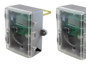
The HLP is used to measure positive, negative or differential pressure. The piezoresistive sensor is ideal for monitoring the pressure of air or other clean inert gas. Typical HVAC applications include monitoring of filter differential pressure or VAV applications. An integrated static pressure probe provides ease of installation for duct mounting. Several accessories are available. A weatherproof polycarbonate enclsoure is provided for electrical connections and ease of installation.
